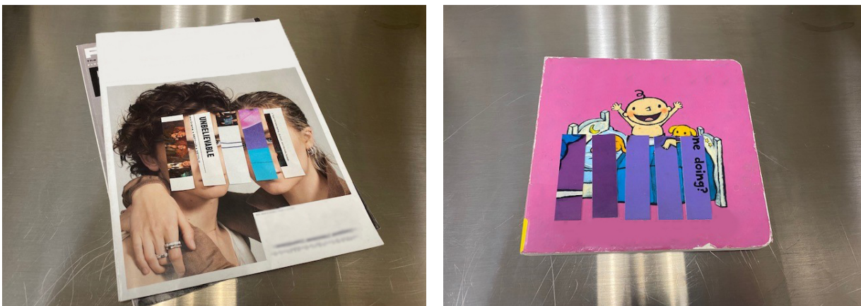
Figure 1. Inoculation of SARS-CoV-2 onto test materials (magazine—left; children’s board book—right). After the inoculation, the extracted test coupons were placed back inside the closed item.
