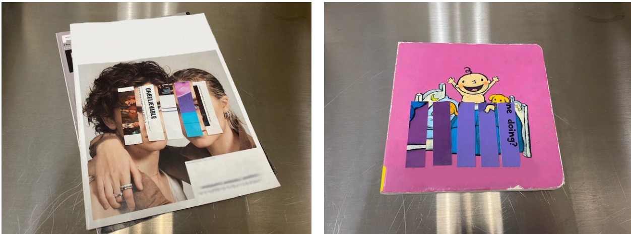
Figure 1. Inoculation of SARS-CoV-2 onto test materials (magazine–left; children’s board book–right). After the inoculation, the extracted test coupons were placed back inside the closed item.
