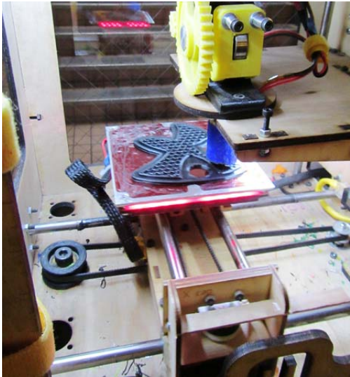
A honeycomb layer is laid down.
